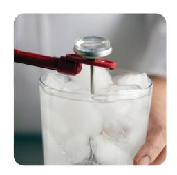
2. Submerge the sensing area, and wait 30 seconds.
