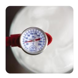
3. Adjust the thermometer so it reads 32°F (0°C).
